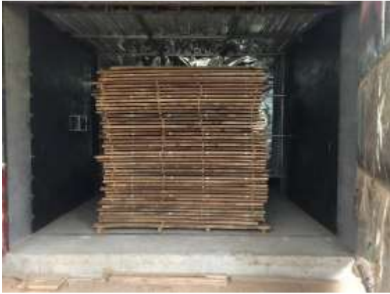
Figure 16: Installation of baffling in Mr Niphone's kiln in Luang Prabang (left: before baffles were installed, right: timber stack with baffles installed)
