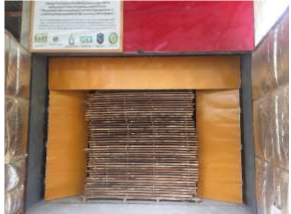
Figure 16: Installation of baffling in Mr Niphone's kiln in Luang Prabang (left: before baffles were installed, right: timber stack with baffles installed)
