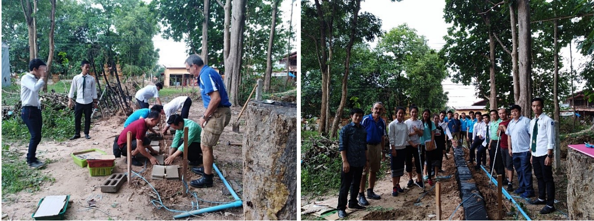
Figure 15: FoF students and researchers participate in establishing long term termite and fungal durability trials
