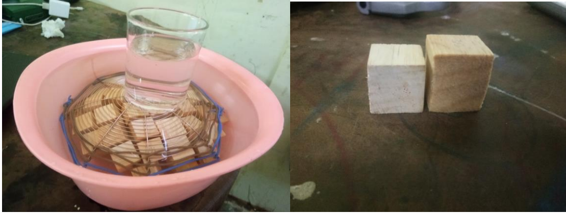
Figure 06: Water absorption and dimensional changing experiment.
