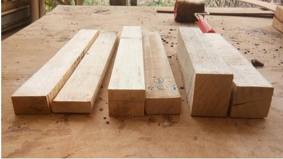
Figure 05: Comparison the dimension of the control wood and densified lumbers
