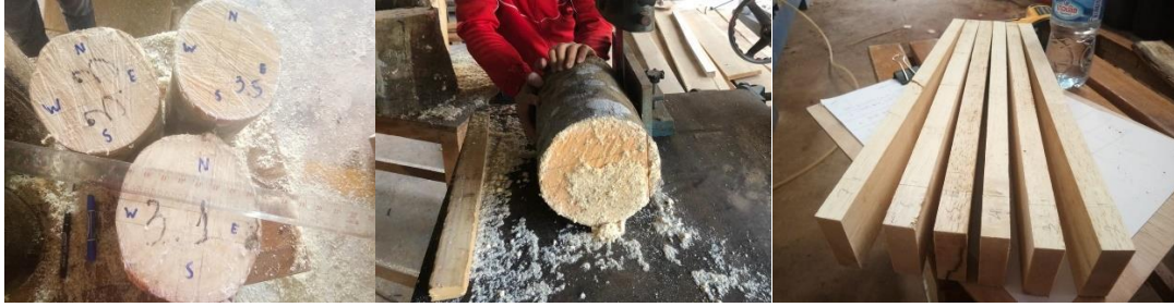
Figure 01: Log breakdown designing and sawing
