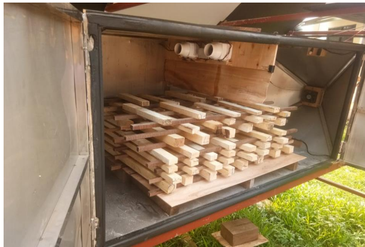
Figure 03: Drying Rubber wood by Solar kiln
