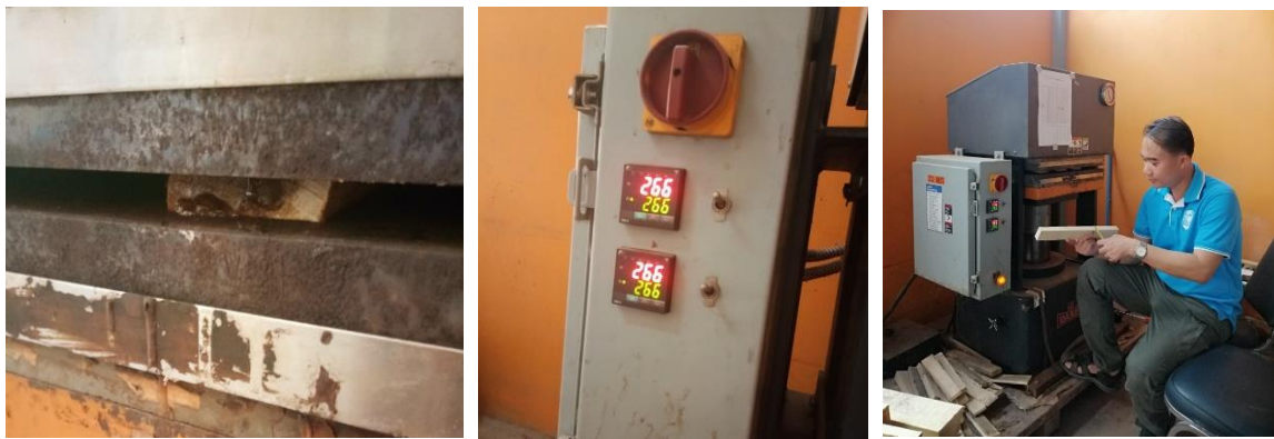
Figure 04: Wood densifying by a hot press machine
