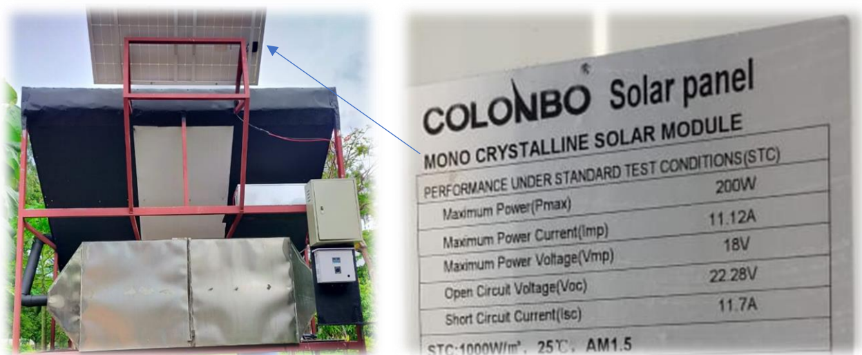
Figure 7. Solar panel's specification
