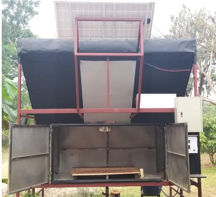
Figure 2. Front view of a solar kiln
